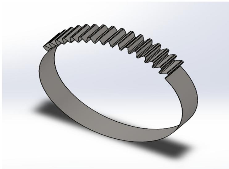
Figure 9.Coating layer modeled for gears
