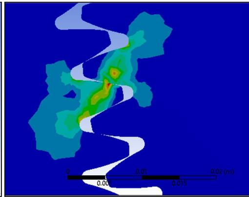
Figure 7. Stress plot at contact region
