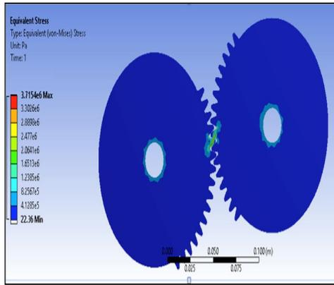
Figure 6. Stress plot for non-coated gears
