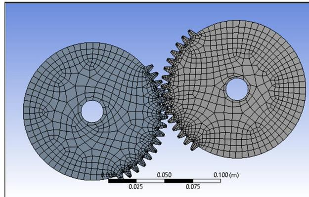
Figure 4: Meshing applied to pair of gears
