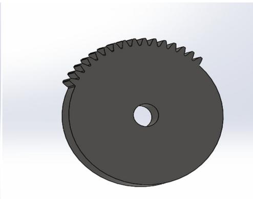
Figure 2. Gear with few teeth modelled
