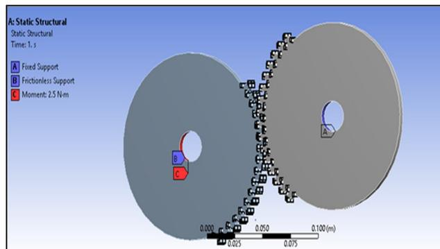
Figure 5. Boundary conditions applied on gear pair
