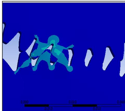
Figure 11. Stress at the contact region for coated gears
