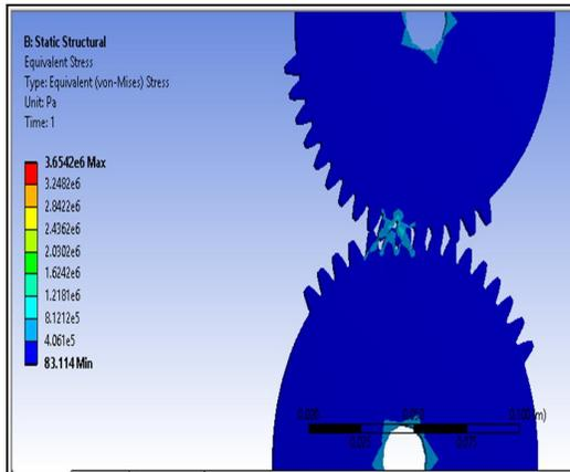
Figure 10. Stress plot of Coated Gears
